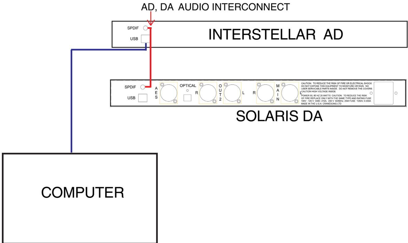
By using the AD as the master interface the clocking will be uncompromised
