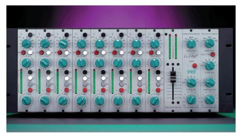
preamp — gain blocks which were designed to exhibit warm sound and excellent transient response. Each Spider input channel also incorporates a switchable "fat" amplifier stage, in order to supply tube-like color upon demand. This analog circuit is modeled after the one used in Crane Song's Flamingo mic-pre. The mixer can be switched to eight channels of line input (on 1/4-inch phone jacks) as well.
