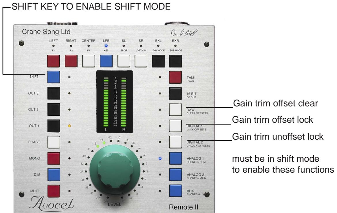
Gain trim can be cleared, locked or enabled by using the Shift key to reach the desired selection.
