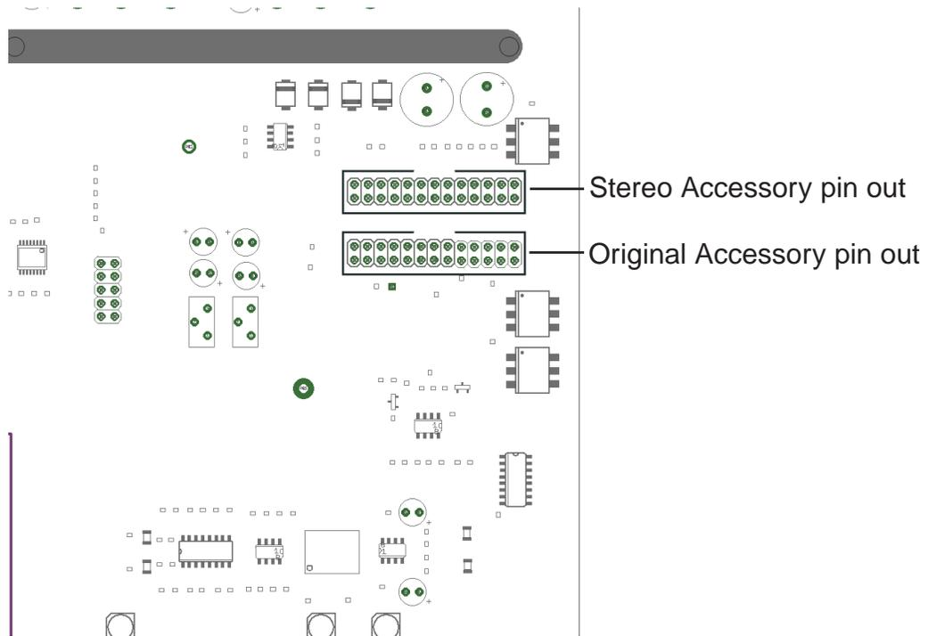
Avocet IIA shipped configured for stereo will have the Accessory connector configured in the stereo mode. This uses the Tascam style of signal assignment. Any one who upgrades from an earlier version and uses the Accessory connector may need to move the internal ribbon cable
