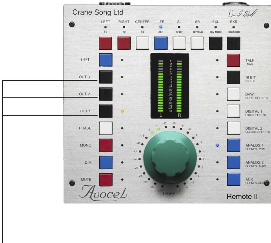
By pressing all three output selection buttons at the same time Avocet will reset all of its internal settings. This is the same as rebooting the remote.
