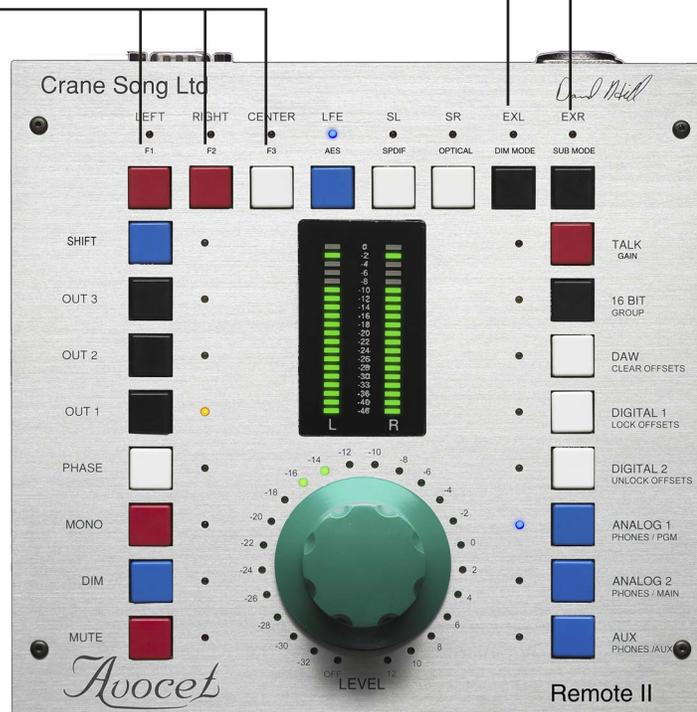
The OUTPUT LEVEL of each speaker may be trimmed down for speaker level matching. When setting up the system so that the normal listening level is around 0 on the dial. When entering the speaker / output setup. No reduction in level is indicated with the level leds showing 0. The speaker trims are in 0.25 db for a max trim of -15.75db. There are 4 steps per db or 8 steps to get to the -2 setting on the dial.
