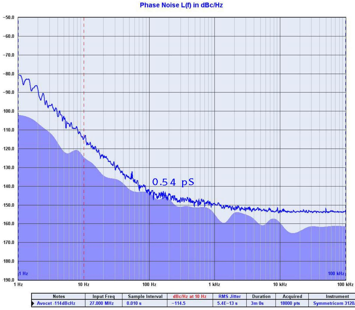
The jitter value in this measurement from 1Hz to 100KHz is 0.54pS typical measured with a Symmetricom 3120A using a Stanford Research Systems Rubidium Frequency Standard, PRS10
