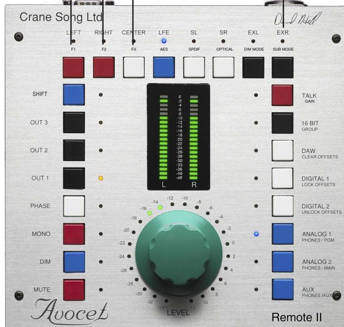
The OUTPUT LEVEL of each speaker may be trimmed down for speaker level matching. And setting up the system so that the normal listening level is around 0 on the dial. When entering the speaker / output setup, no reduction in level is indicated with the level LEDs showing 0. The speaker trims are in 0.25 db for a max trim of -15.75db. There are 4 steps per db or 8 steps to get to the -2 setting on the dial.
