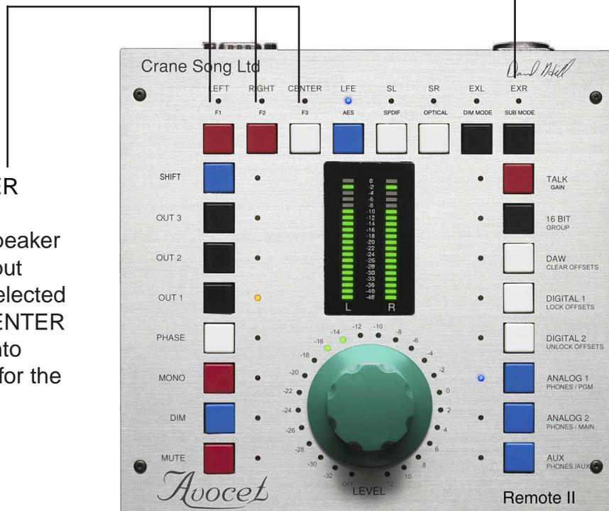
The OUTPUT LEVEL of each speaker may be trimmed down for speaker level matching
