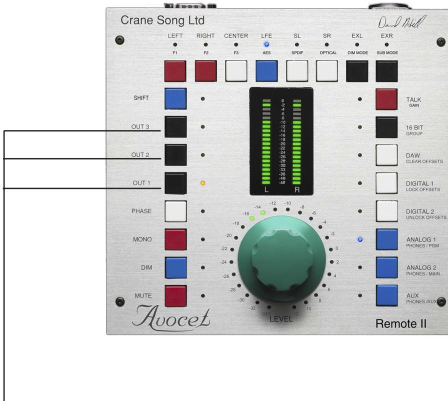
By pressing any one of the speaker select buttons a second time and holding it for about 0.5 seconds will put Avocet into the speaker set up mode.
